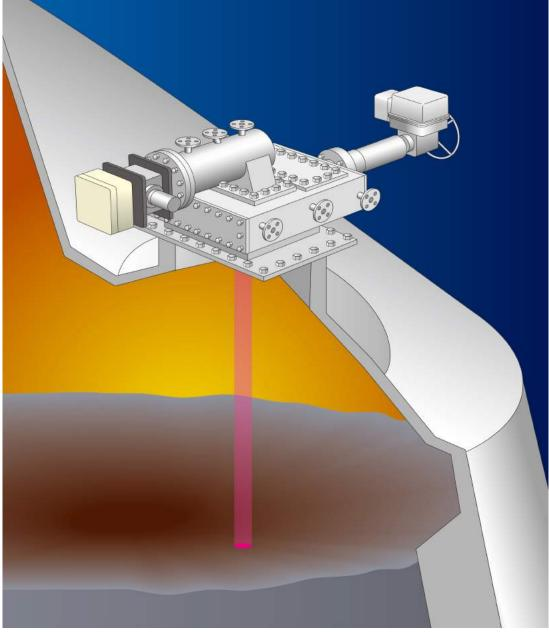
The Wadeco MWS-BF-2D Milli-Scanner is a combination of a mechanical scanning system and high-speed rangefinder which can be used to display a 2D stockline profile after every feeder rotation.
