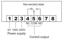
\* Phase of power supply must be same from both transmitter and receiver.
